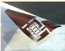
Fig. 1: Example of an inkjet printed circuit
