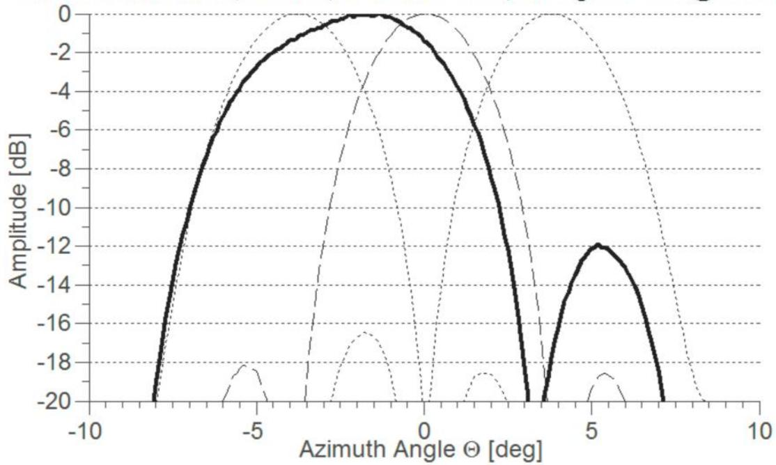
Relative amplitudes of example antenna recombination pattern (solid) with a high gain at -2 degrees offset direction and a null close to +3degrees offset direction. Angle in azimuth direction and amplitude as relative gain measurement.
