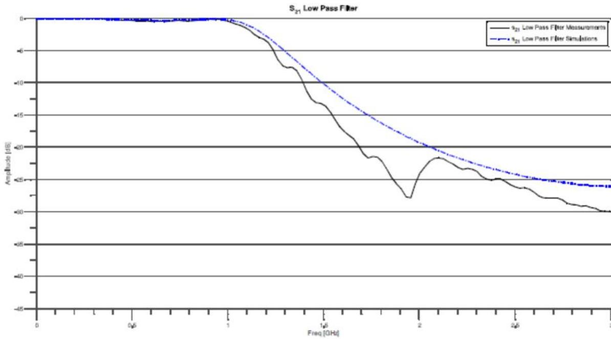
Band pass filter, S<sub>21</sub>. Measurements (black) vs Simulations (blue)
