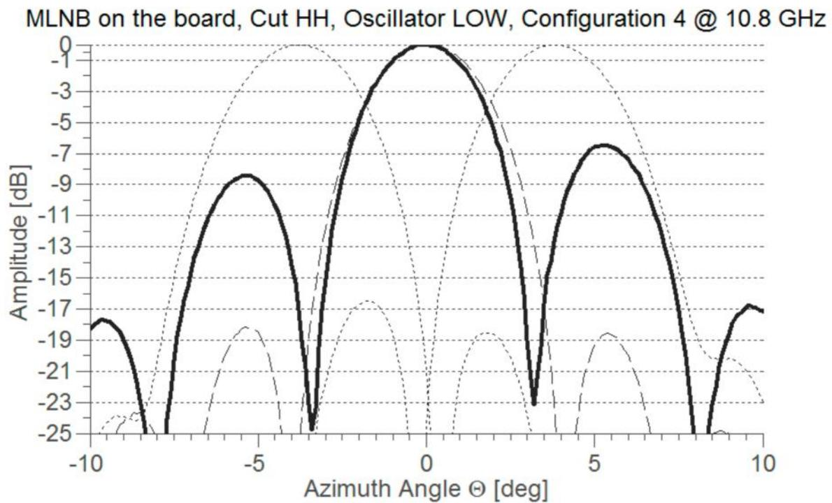
Measured recombination gain pattern example configuration over azimuth angular direction at 10.8GHz. The solid line is an example beamforming recombination of a narrow beam with nulls close to +3 degrees offset.
