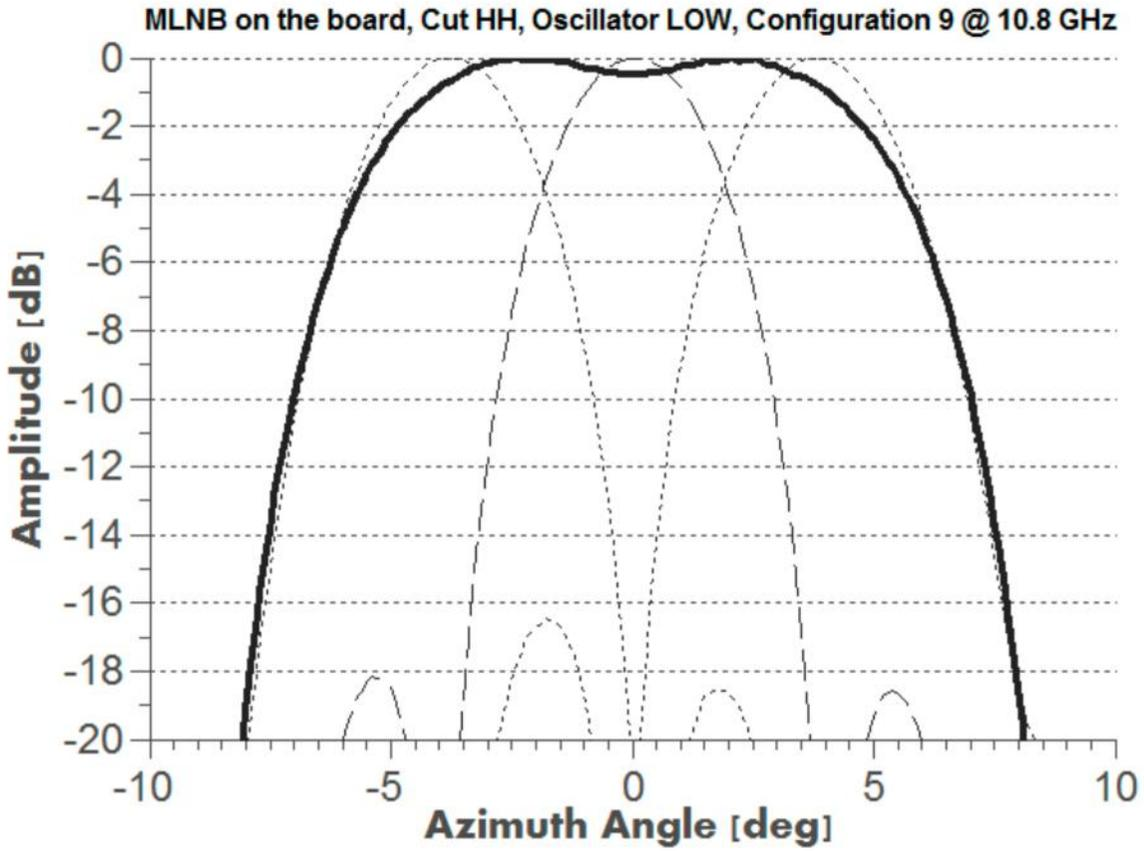
Measured example relative beamforming recombination pattern with a high gain over the entire azimuth field of view and compared to the individual 3 feed gain patterns (dashed line). The amplitude is a relative measurement and the angle is in azimuth direction.
