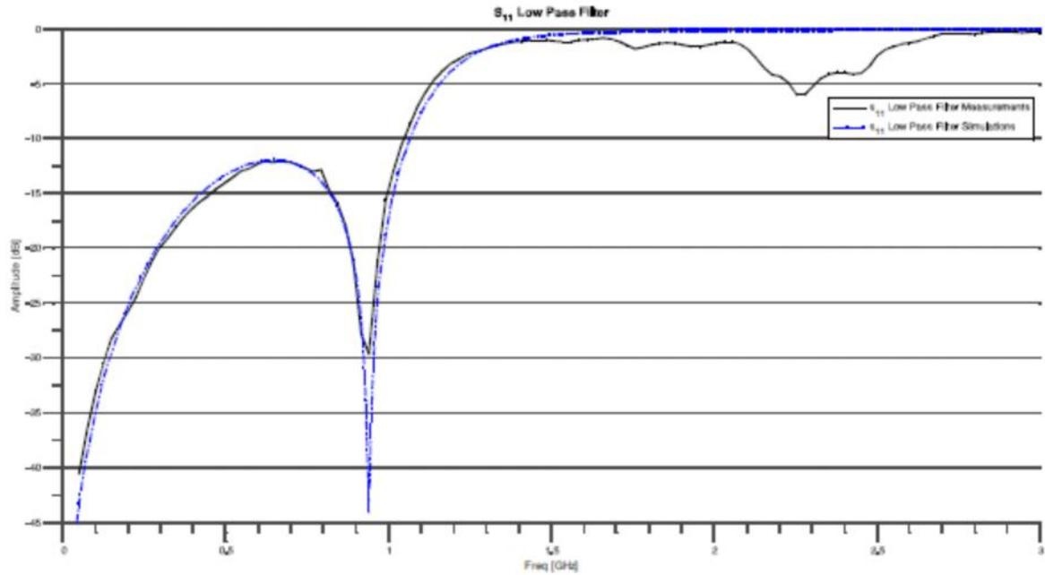
Low pass filter, S<sub>21</sub>. Measurements (black) vs Simulations (blue)
