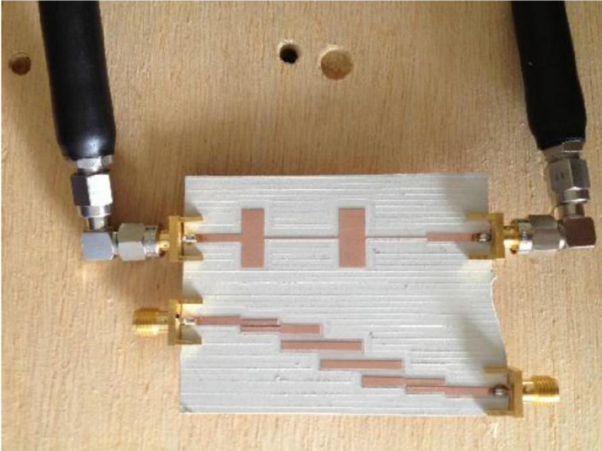
Fabricated RF low pass filter (above) and band pass filter (below) on duroid substrate.
