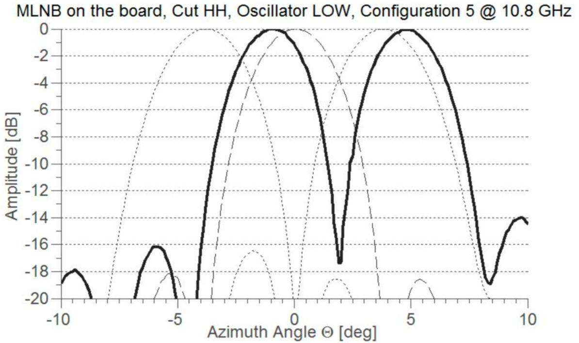
Relative amplitudes of an example antenna recombination pattern (solid) with a specific null at +2 degrees offset.
