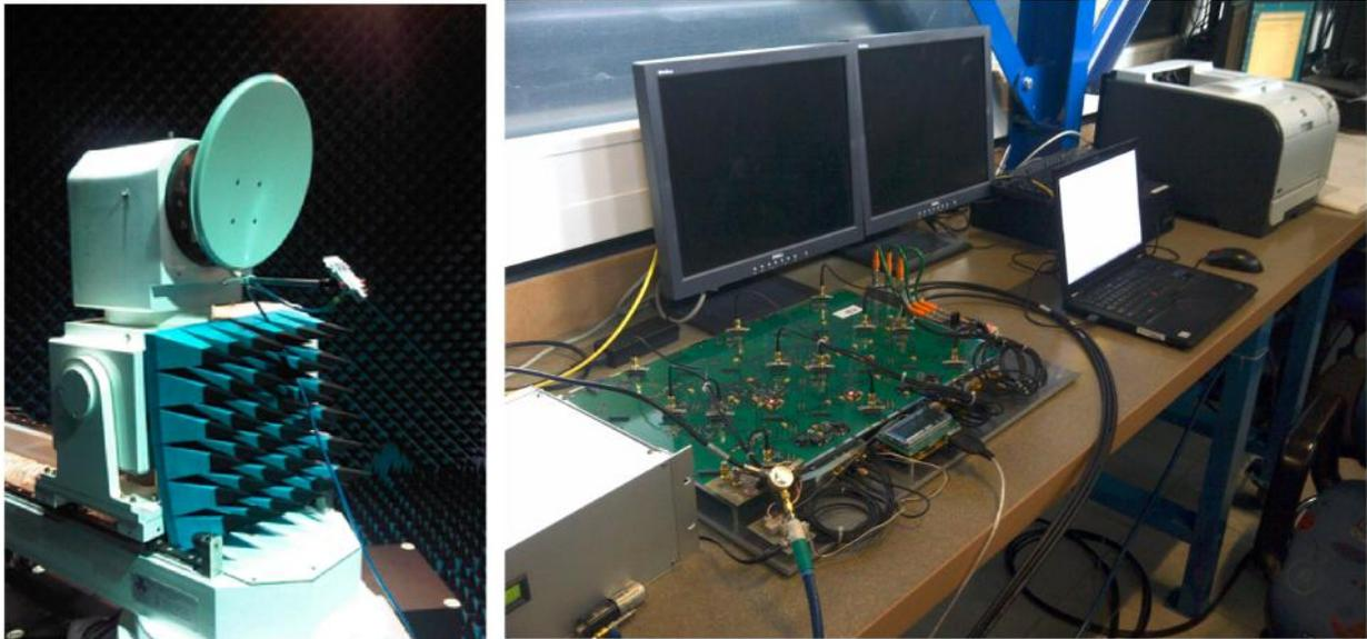
Picture of the MLNB demonstrator antenna in the anechoic chamber at the compact antenna test range (CATR) at ESTEC, Noordwijk. The board beamforming hardware demonstrator is on the right.
