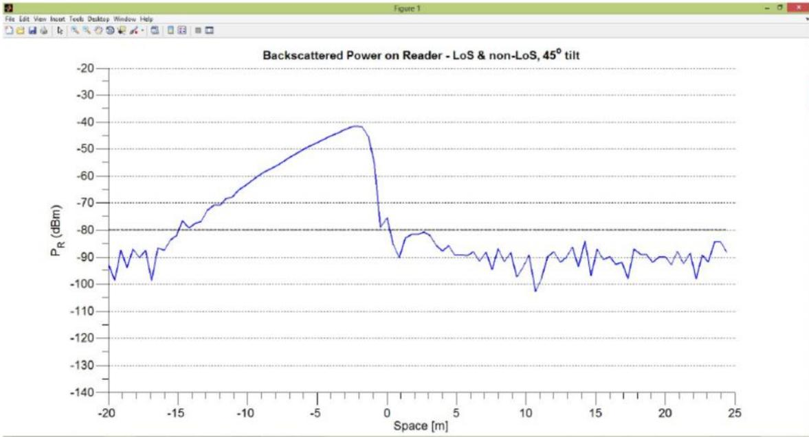
Example of a simulation output: received power level from the antenna mounted on the moving vehicle and at variable distance from the receiver.
