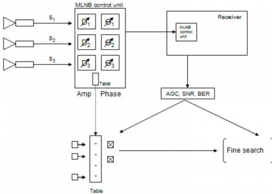
Setup of the beamforming demonstrator. Illustration of the beamforming setup with the receiver and signal quality metrics (AGC, SNR, BER) for fine pointing.
