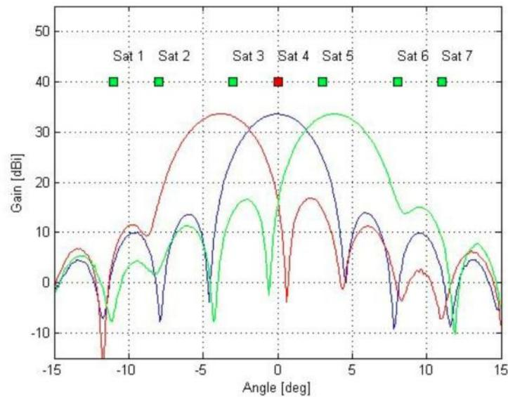
Azimuth cut of the simulated beam gain patterns for the prototype and illustration of a possible reception scenario with Sat3, Sat4 and Sat5 within the field of view of the receiver.
