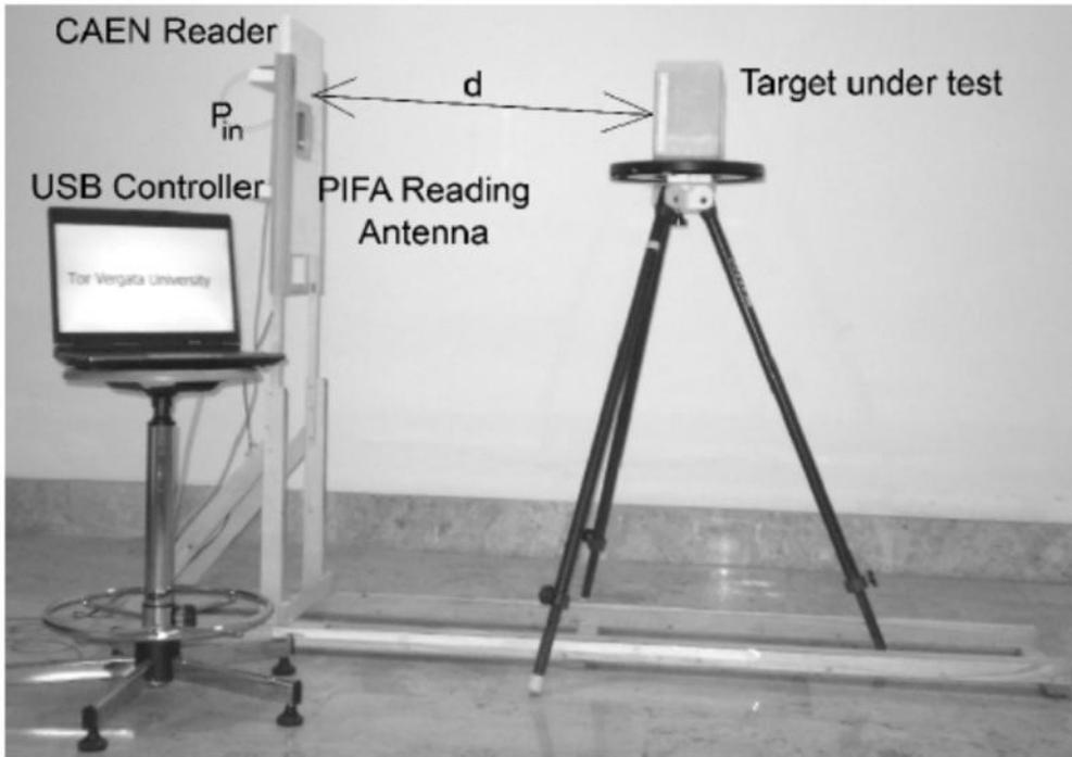
Measurement set-up comprising a low-range reader, a PIFA linear polarized antenna and a computer controller.
