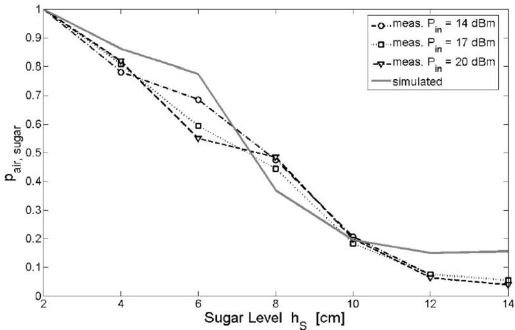
Sugar box: Normalized simulated and measured backscattered power for the multi-chip system which is monitoring the sugar level inside the box. The measurements have been repeated for some input powers.
