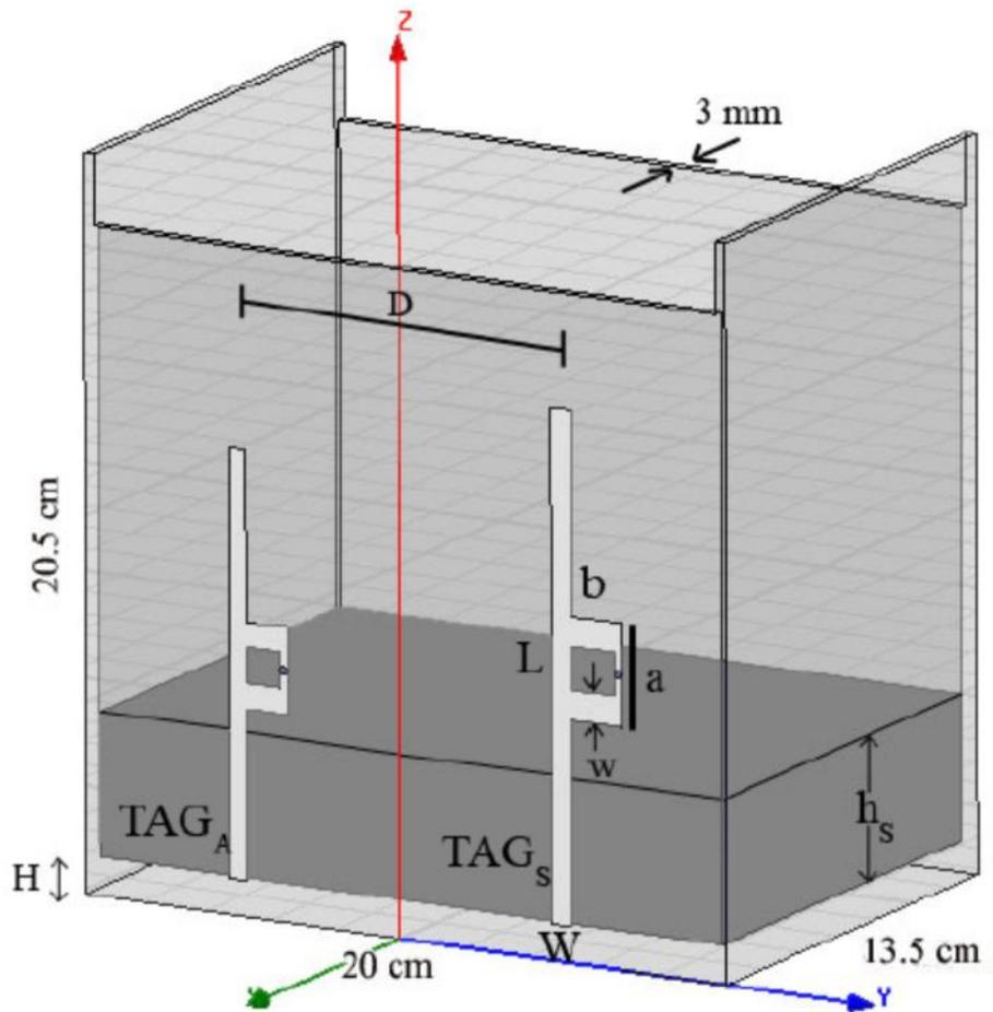
Passive tags to sense the level of sugar powder within a perspex box. Geometrical size (in [mm]):  $H=12$ ,  $D=95$ ; TAG<sub>S</sub>  $L=142.8$ ,  $W=6$ ,  $a=28.8$ ,  $b=15.6$ ,  $w=8.4$ ; TAG<sub>A</sub>  $L=119$ ,  $W=5$ ,  $a=24$ ,  $b=13$ ,  $w=7$ .
