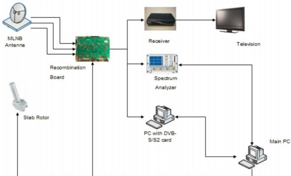
Demonstrator setup in the lab with connected test and measurement PC with DVB-S/S2 card and reception chain for broadcast reception in parallel. Tests over azimuth pointing angles are automated with a conventional Stab motor.
