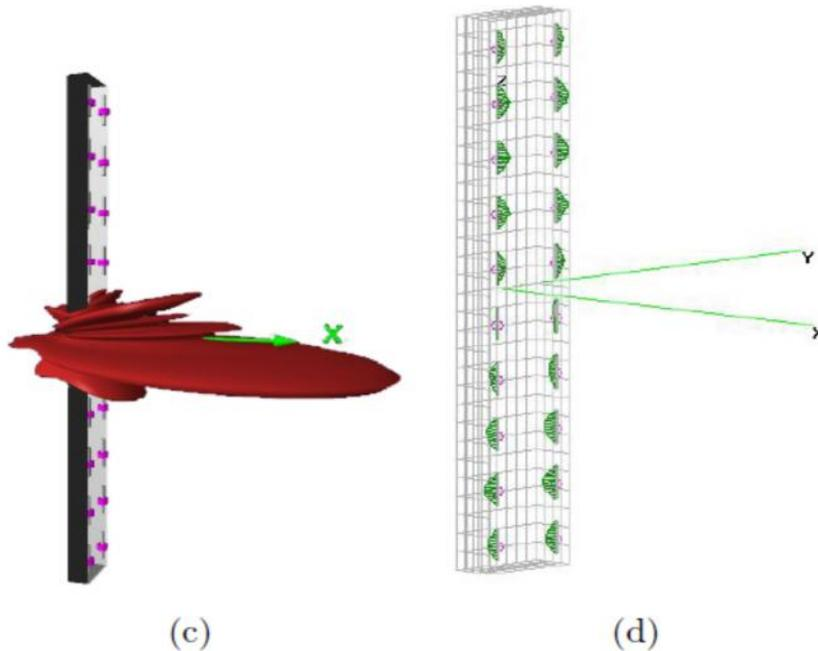
Radiation diagrams of a) Vertical plane and b) horizontal plane for an array uniformly excited. Tridimensional representation of c) the array antenna pattern and d) the array element position in the radome.
